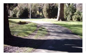
Figure 3: Sharp curves combined with poor sight distance
