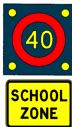
Figure 14. A 40 km/hr school zone option (from Traffic Note 37) that may be appropriate for some rural schools with significant pedestrian risk, if the surrounding speed limit is already lower (e.g. 80 km/hr) and environmental cues reinforce school activity.
