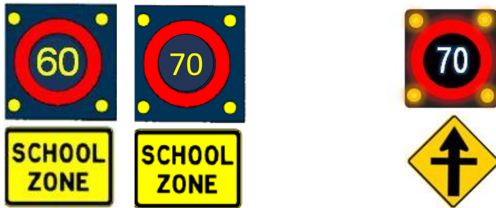
Figure 13. Possible active mandatory speed reduction signs to reduce the risk of side impact serious harm, for school (left) and intersection (right) contexts. For school environments, a 70 km/hr sign would be used within a permanently signposted 100 km/hr environments, whereas the 60 km/hr version would be used within permanently signposted 80 km/hr environments.
