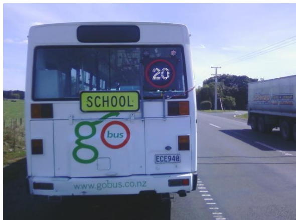
Sign A. Small sign, reflective red circle around illuminated number
