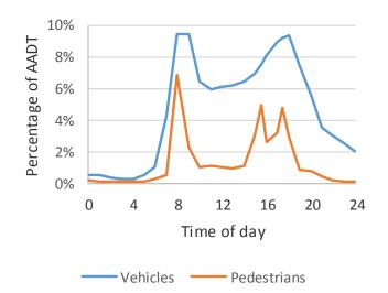
Figure 10: Hourly flow profiles for pedestrians and vehicles
